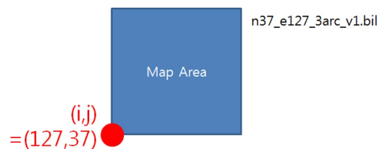
Fig. A4. Longitude and latitude values in the SRTM file name (n37_e127_3arc_v1.bil) and their actual location in the SRTM data.
