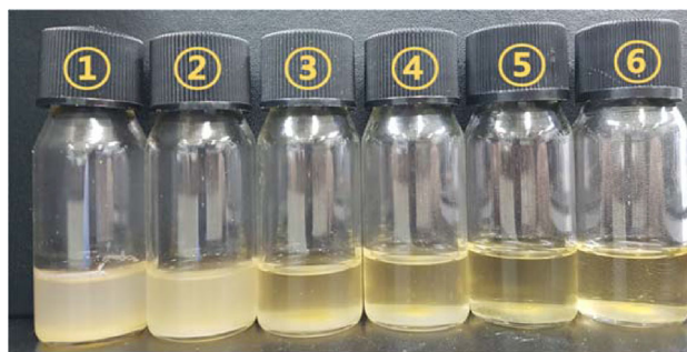
Fig. 1 The appearance of the mixture of rosemary extract (1000 ppm) and tween 20 solutions (①: 0%, ②: 0.1%, ③: 0.5%, ④: 1%, ⑤: 2%, ⑥: 4%)
