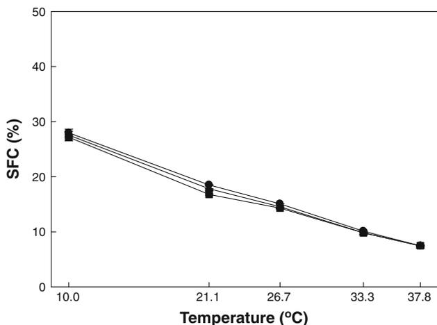
Fig. 5 SFC (%) of the interesterified oils in the single- (filled circle), double- (filled triangle), and triple-stage (filled square) PBER systems
