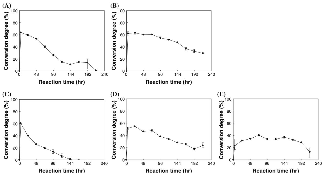
**Fig. 4** Conversion degrees of the first (a, c), second (b, d), and third (e) reactors in the double- (a, b) and triple-stage (c–e) PBER system at 38.2 % FHCO in blended oil at a 0.4 mL/min flow rate. The
