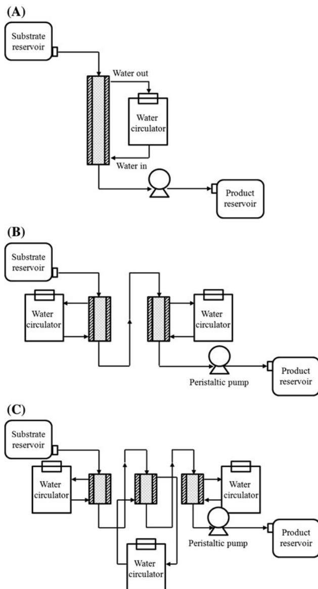
**Fig. 1** Schematic diagram of single- (a), double- (b), and triple-stage (c) PBER system for the production of interesterified oils
