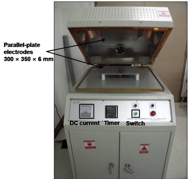
Fig. 1. Radio-frequency (27.12 MHz) heating system at Seoul National University (Seoul, Korea).
